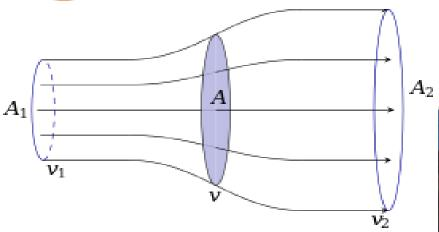
Schematic of fluid flow through a disk-shaped actuator. For a constant density fluid, cross sectional area varies inversely with speed.
