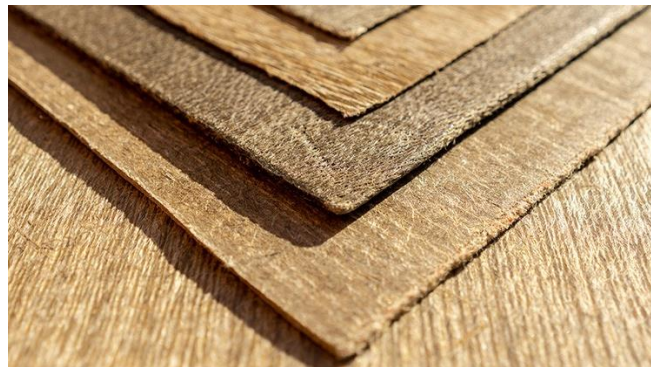
Figure 11 Prepreg layers with PLA and flax fibers, as a green composite.
