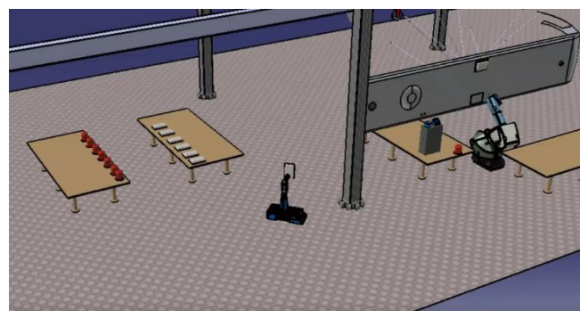
Figure 12 Process of transporting an air condition unit to the assembly area by the mobile robot
