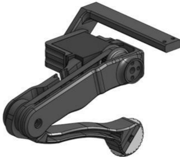
**Figure 3-2 3D representation of Spot Mini Mini's leg structure**
