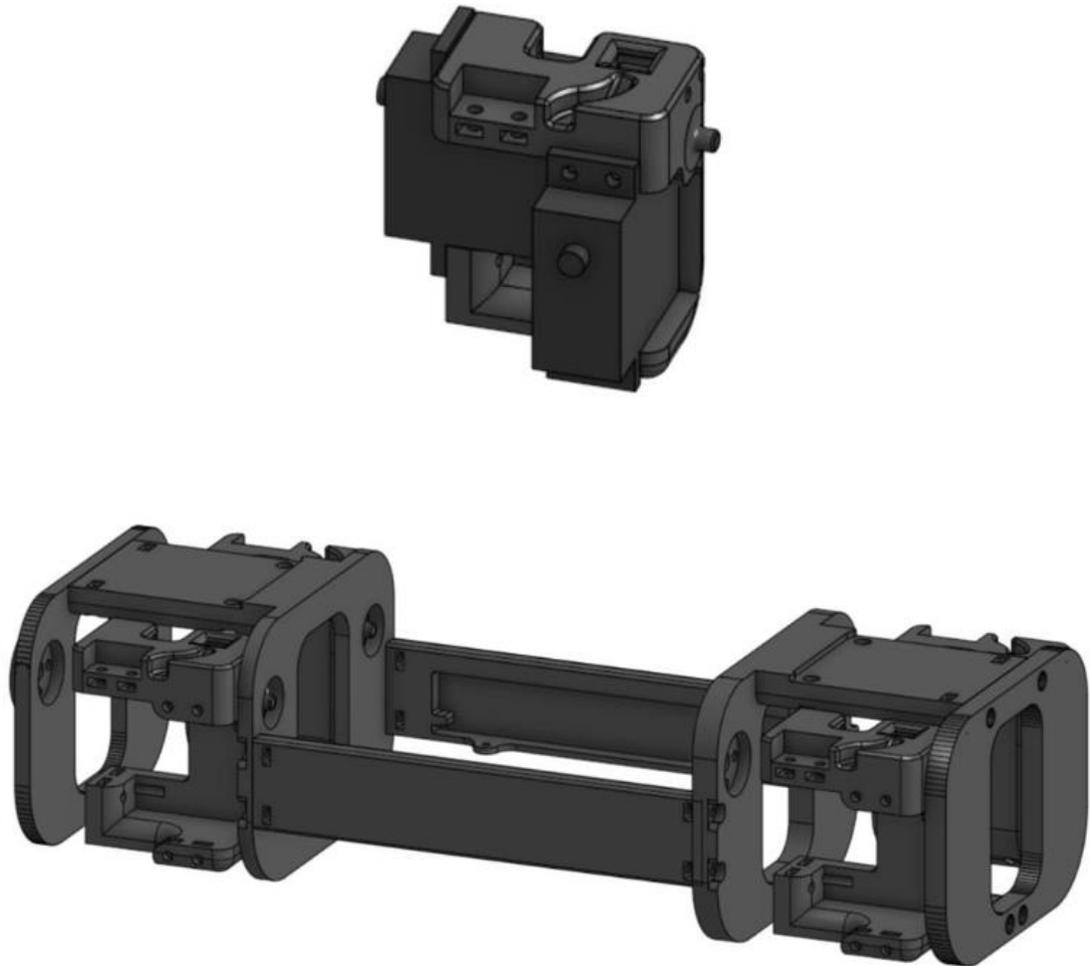
**Figure 3-6 (Above) Hip Joint component of Spot Mini Mini (Bellow) Body structure and hip joint components of Spot Mini Mini**
