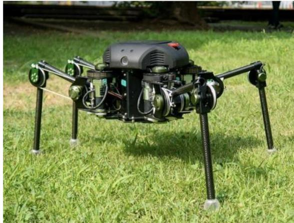
**Figure 2-5** Sprawling type quadruped TITAN-XIII [16]
